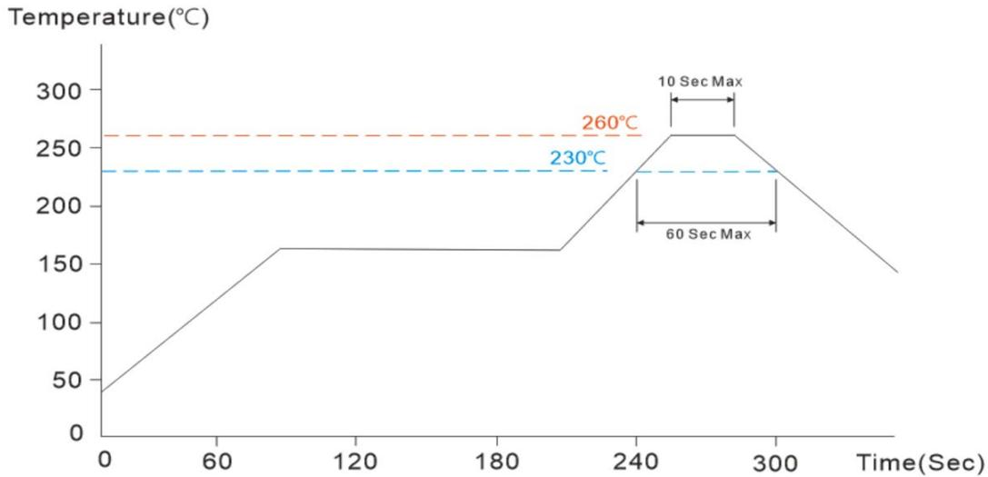
No mechanical and electrical defects are found after testing based on the above profile and keeping under the conditions of room temperature and humidity for 2 hours.
