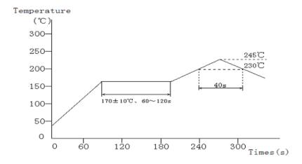
The recommended reflow profile is based on the testing instruments used. Solder ability will depend on the testing equipments, reflow conditions, testing method, etc. So it is necessary to make a confirmation of them when the reflow conditions are set up.
