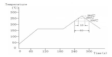
No mechanical and electrical defects are found after testing based on the above profile and keeping under the conditions of room temperature and humidity for 2 hours. Twice reflow test is acceptable with the test interval remaining 1 hour under the normal conditions.
